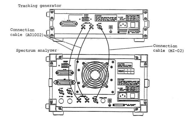
Figure 1-3 Connections between Rear Panels
