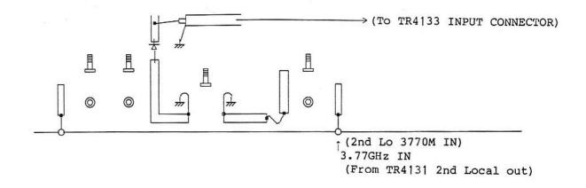
Figure 7-1 Adjustment of 3.77 GHz BPF and ISO Cavity
