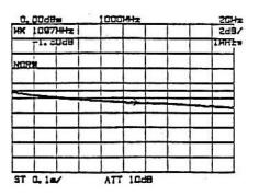
Figure 2-13 Reading Deviation from Reference Line According to Marker To modify or terminate setting after measurement, press and to return to the normal mode.
