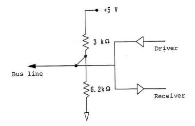
Figure 3-2 Signal Line Termination
