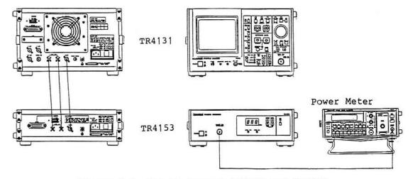
Figure 7-5 How to Connect TR4153 and TR4131
