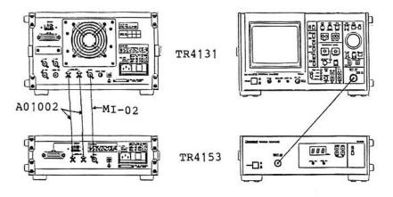
Figure 6-1 How to Connect Cables
