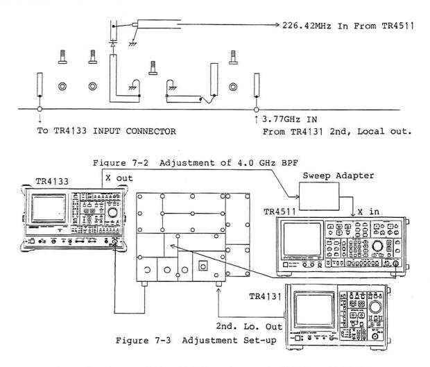
Set up as shown in Figures 7-2 and 7-3. Then, set TR4133 and TR4511 as follows.
