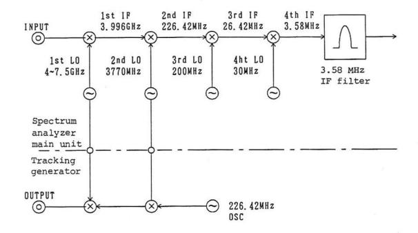
Figure 5-1 Operation Principle Block Diagram
