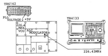
Figure 7-4 Adjustment of 226.42 MHz VCO
