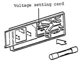
Figure 1-2 Fuse Replacement and Voltage Setting Card
